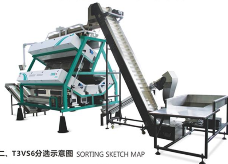
TS-V型三层茶叶色选机 THREE-DECKED COLOR SORTER
